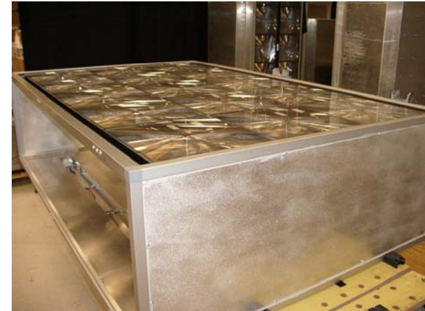
Gen-III CPV Module – 15 1x1 cm 2 CPV solar cells integrated with 1,090X Fresnel lens, producing 450W power
