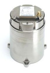
0.5 milli-g in-run bias stability and low VRW ( $80\mu g/\sqrt{Hz}$ .), plus high speed digital signal into a tightly coupled GPS-aided Inertial Navigation System for tactical navigation and geo-location applications.
